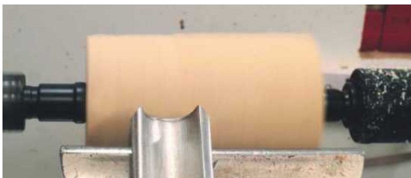
▲ Pic.5 I like to use the tool presented at right angles and use the centre of the tool to turn away the square corners of the wood
